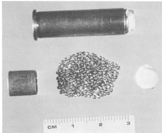
FIG. 1—Glaser Safety Slug opened to demonstrate load. The copper cup is to the left, the plastic plug to the right, and the shot in the middle. An intact round is shown above the slug. (AFIP Neg 78-4650-1.)
