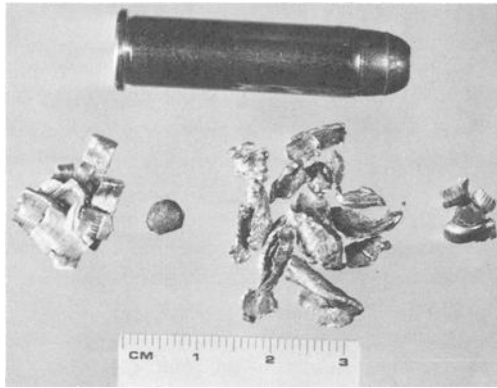
FIG. 7—Recovered Velex/Velet exploding bullet showing (from left to right) the deformed jacket, the No. 4 shot, the fragmented bullet, and the deformed percussion cup. (AFIP Neg 78-4650-7.)
