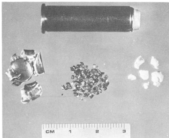
FIG. 4—Recovered Glaser Safety Slug showing deformity of copper cup and shot fragmentation of plastic plug. (AFIP Neg 78-4650-4.)
